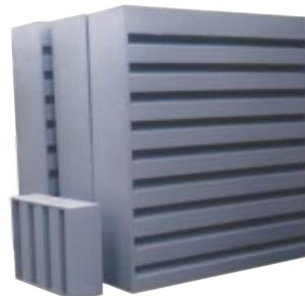
Acoustic louvre available in depths of 300 & 600mm with 100mm or 200mm thick splitters to provide a wide range of acoustic & flow performances.
